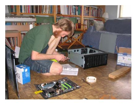
Get out the motherboard. Place the motherboard I/O shield into the slot in the case.
