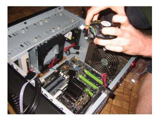
Attach the CPU heat sink.
