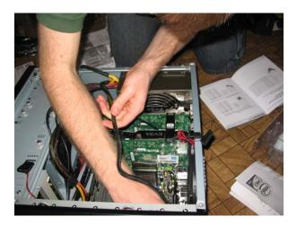
Put in the optical drives, and attach the data cables to the motherboard, and the power cables to the power supply.
