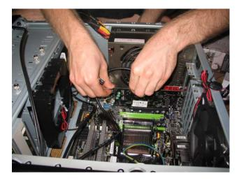
Attach the wires from the case to the motherboard.
