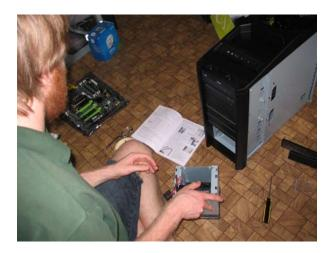
Put the hard drives into their bays, and attach the data cables to the motherboard, and the power cables to the power supply.
