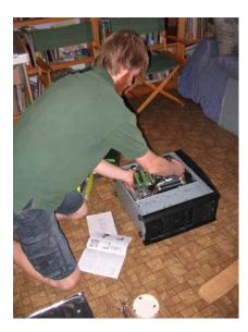
Align the motherboard holes with the standoffs and screw it in.
